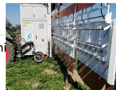
**Strong points**: Fairly large width of intervention per passage (9 to 12 m) allowing a significant work output – Intervention possible even in wet soil conditions – Significant impact on immature vegetation without physical destruction of the tops – Reinforced action on crushed tops.
